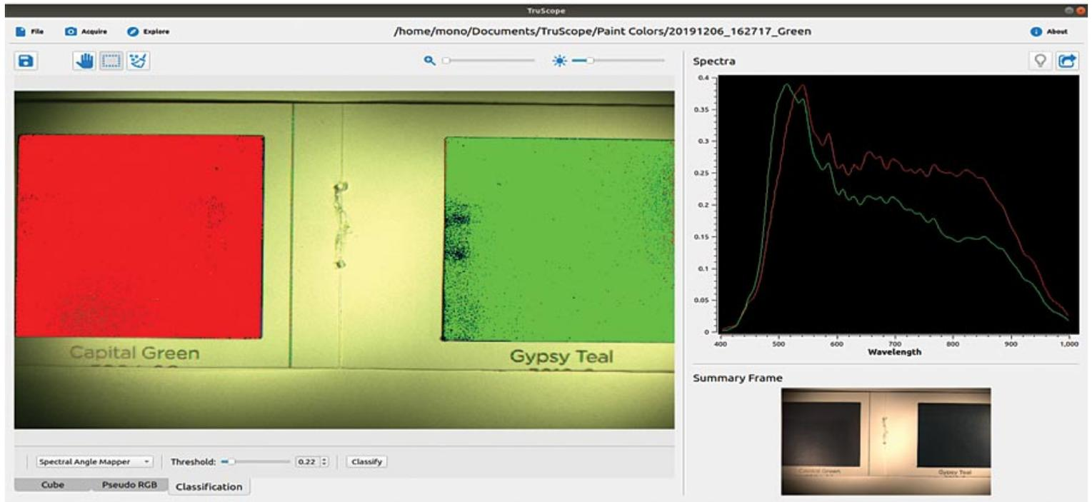
*This image shows the Spectral Angle Mapper classification of paint samples, demonstrating detection of the differences between otherwise indistinguishable pairs of greens (capital green and gypsy teal). The sample as they would appear to the human eye are in the bottom right corner.*
