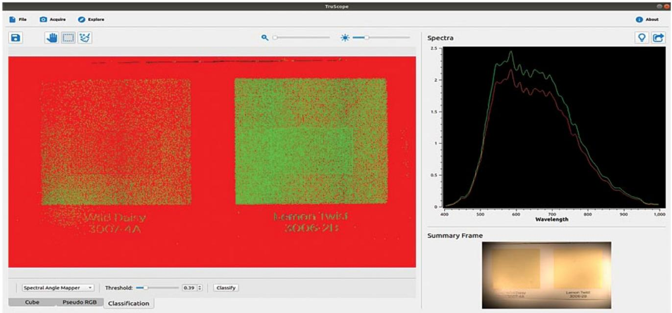
*This image shows the Spectral Angle Mapper classification of paint samples, demonstrating detection of the differences between otherwise indistinguishable pairs of yellows (wild daisy and lemon twist). The sample as they would appear to the human eye are in the bottom right corner.*
