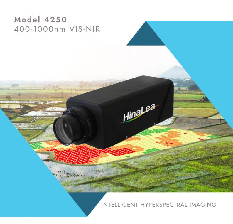
inaLea's 4250 VNIR system represents the next generation of intelligent hyperspectral imagers. Based on front-staring Fabry Perot technology, the 4250 includes hardware and software required to support a broad range of hyperspectral imaging applications. A tunable filter that sequentially selects spectral bands is placed in front of the sensor and generates the hyper-cube by collecting complete images at each spectral band-pass.
